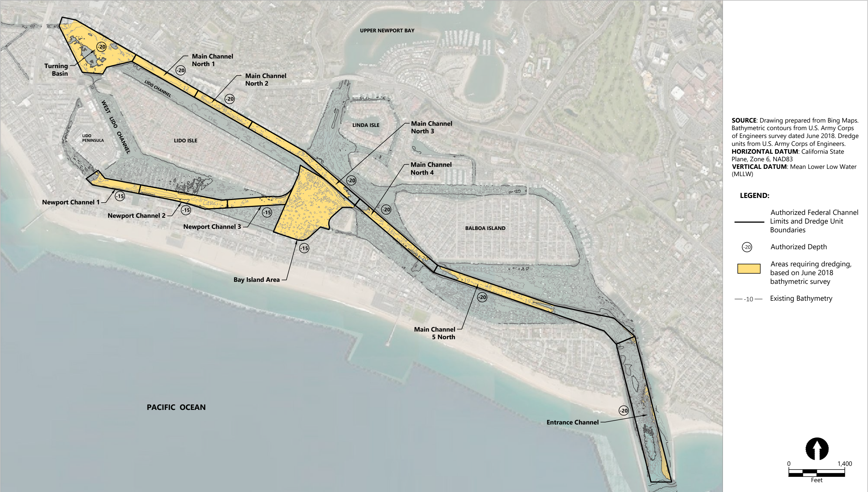
Figure 2 Overview of Authorized Design Depths, Dredge Units, and Bathymetry for Federal Channels Maintenance Dredging Sediment Management Plan Lower Newport Bay
