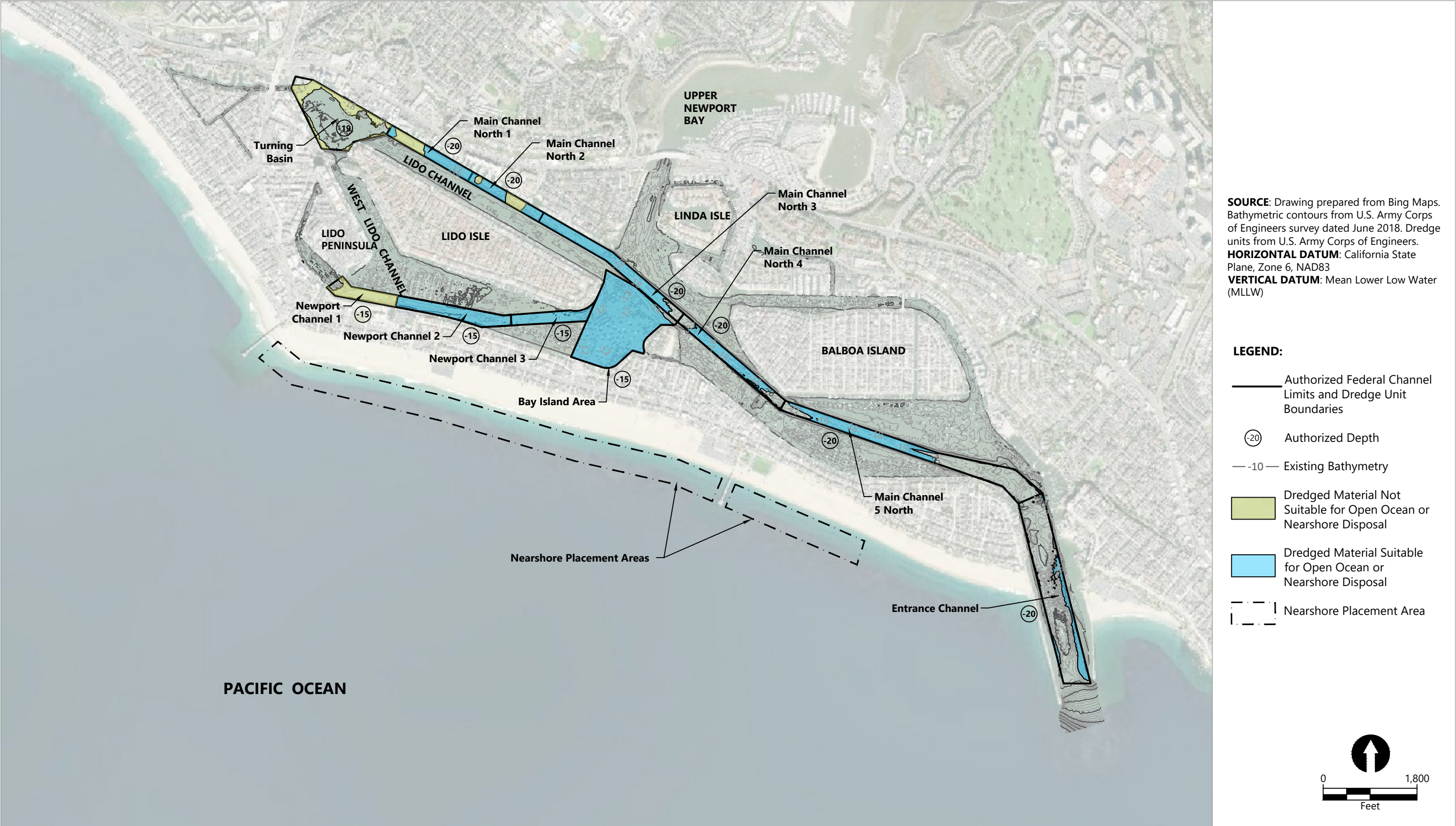
Figure 3 Federal Channels Maintenance Dredging Sediment Suitability Map Sediment Management Plan Lower Newport Bay
